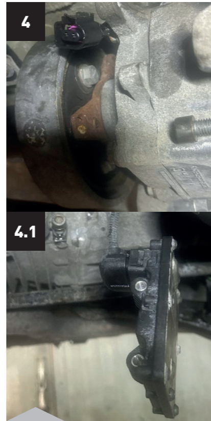
(Figures 4 + 4.1) Disconnect the precharge pump connector between the control unit and the pump. For better access, remove the control unit from its mounting.
